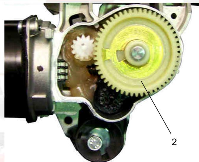
Put the new clip (ref.3) in place on the motor axle, like the original one.
