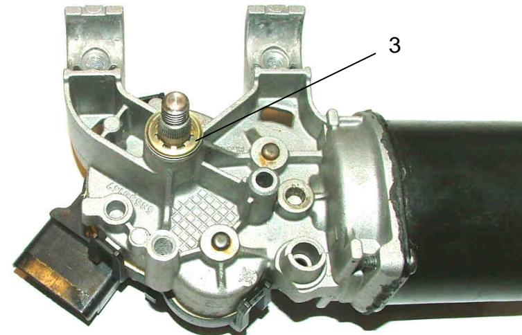
Apply a small strip of silicon seal on the standard seal of the windscreen wipe motor cover (ref. 1), as shown in the photo opposite.
